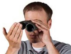
**Adjust the diopter**—start by closing your left eye or covering the left objective lens with your hand. Look through your right eye and adjust the diopter until the object is in focus. Make note of this diopter setting in case you need to set it again.
