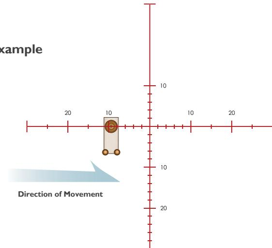
9.4 MOA reticle correction for a target moving 3 mph at a distance of 800 yards. No wind. Total bullet time of flight from trigger pull is 1.5 seconds during which target travels 6.6 feet. Elevation already dialed into turret.
