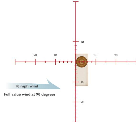
3 MOA reticle windage correction at 400 yards in 10 mph crosswind using center crosshair. Elevation adjustment already dialed into the riflescope.
