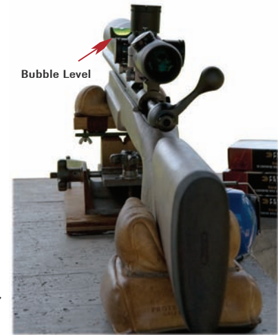
Confirm the vertical orientation of the reticle.
