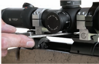
Square the riflescope to the base.
